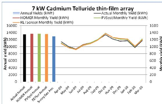
Figure 7: 7 kW CdTe thin-film array results
