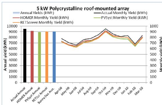
Figure 5: 5 kW polycrystalline roof-mounted array results
