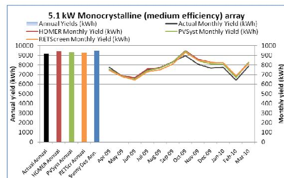
**Figure 2:** 5.1 kW monocrystalline (medium efficiency) array results
