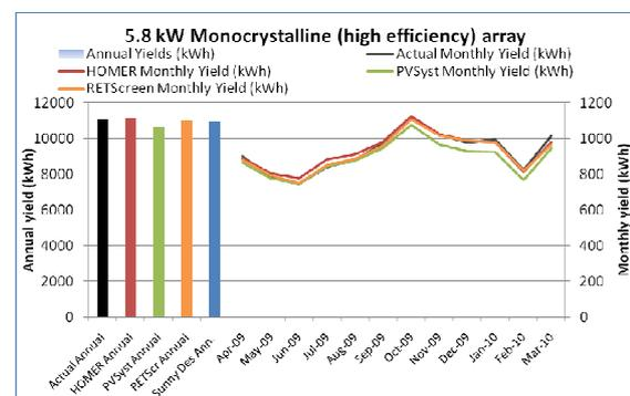
**Figure 3:** 5.8 kW monocrystalline (high efficiency) array results
